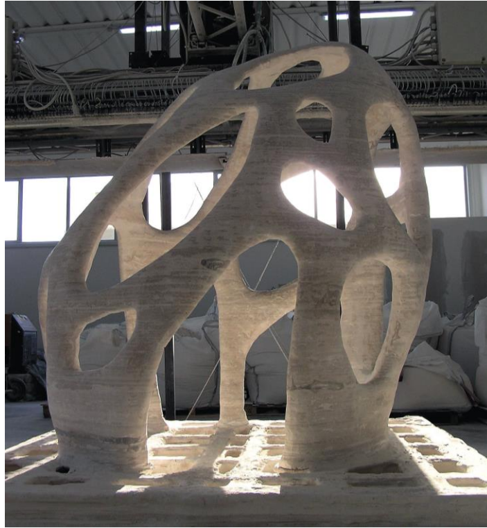
Fig. 29. Radiolaria project, a proof of concept of the D-Shape printer
