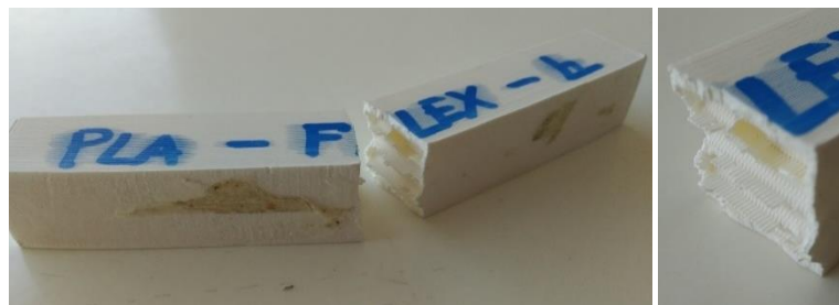
Fig. 29. Part displaying fracture after flexural stress test – strains perpendicular to force: a (left) a typical fracture, b (right) close-up showing infill deformation.
