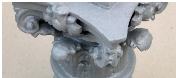
Fig. 10. Part printed with a polyamide, showing finish quality
