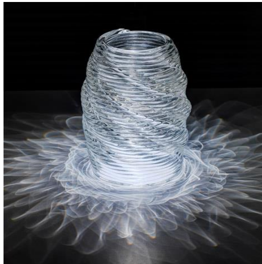
Fig. 14. Vase realized by means of glass printing. Additive Manufacturing of Optically Transparent Glass ( Klein, et al., 2015 )
