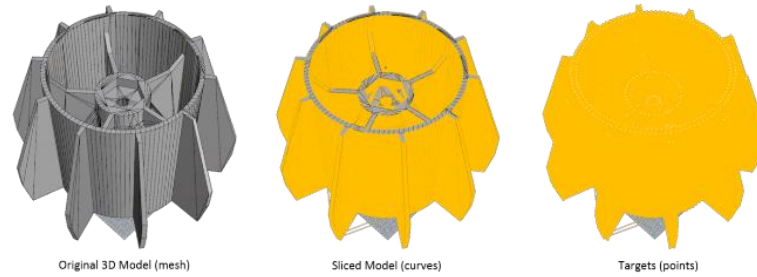
Fig. 7. Internal slicing process and conversion to points
